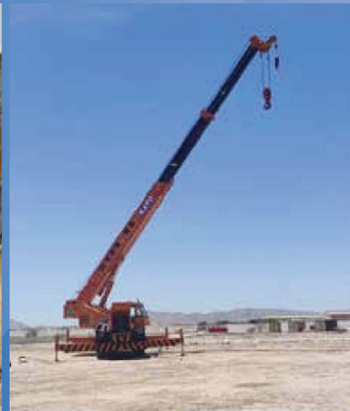
50 TON FOUR WHEEL CRANE
